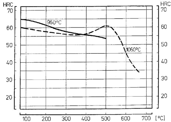
Fig. 11 Influence of temperature on hardness of workpiece material with respect to different tempering temperatures
