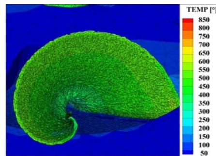
Fig. 5 Chip produced by geometry B
