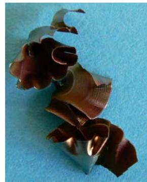
Fig 18 Chip shape produced by real prototype
