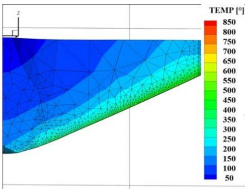
Fig 12 Temperature field distribution on twist drill's rake face
