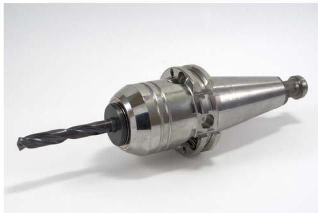
Fig 16: Clamped twist drill
