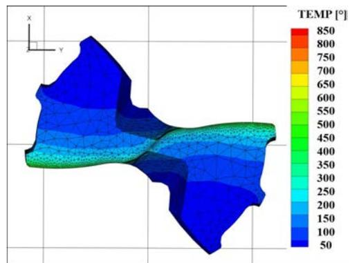
Fig 13: Temperature field distribution on twist drill's flank face
