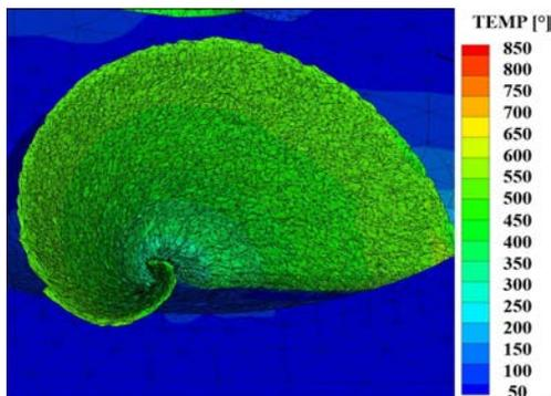
Fig 17: Chip shape predicted by numerical analysis
