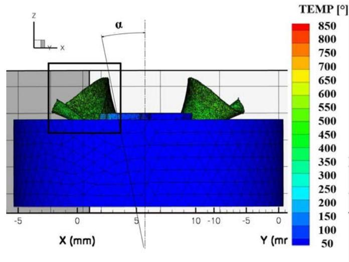
Fig. 6 Inclination angle  $\alpha$  between drill's axis and chip
