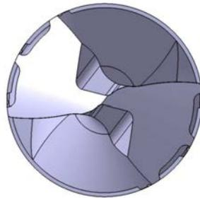
Fig. 1: Model of solid twist drill
