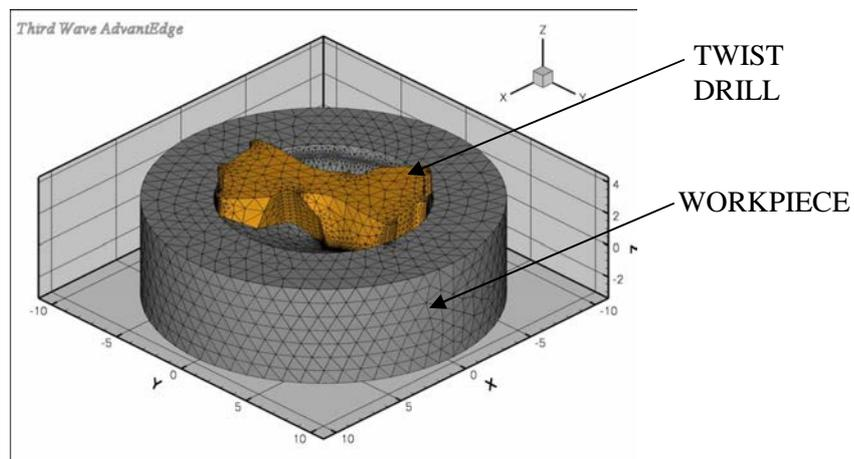
Fig. 3: Meshed twist drill and workpiece
