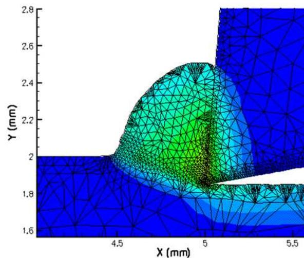
Fig 21 Temperature field distribution in cutting zones
