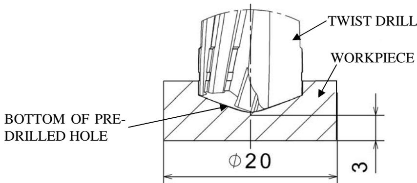
Fig. 2: Computational model of the twist drill and the workpiece
