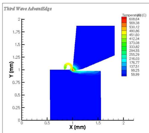
**Figure 4:** Simulation of Temperature for one tooth during the cutting process
