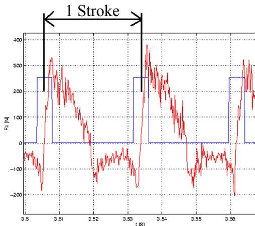
**Figure 3:** Cutting force during one stroke for a test manually controlled
